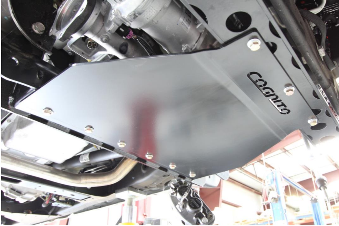
Figure 15: install 1923 skid plate
