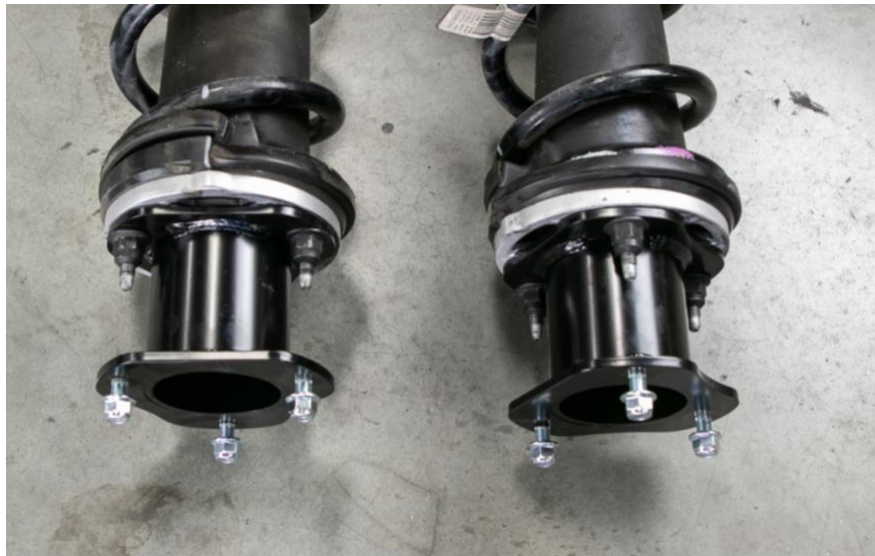
Figure 16: Strut spacers installed on struts
