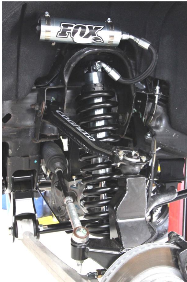
Figure 17: Fox remote reservoir shock mounting
