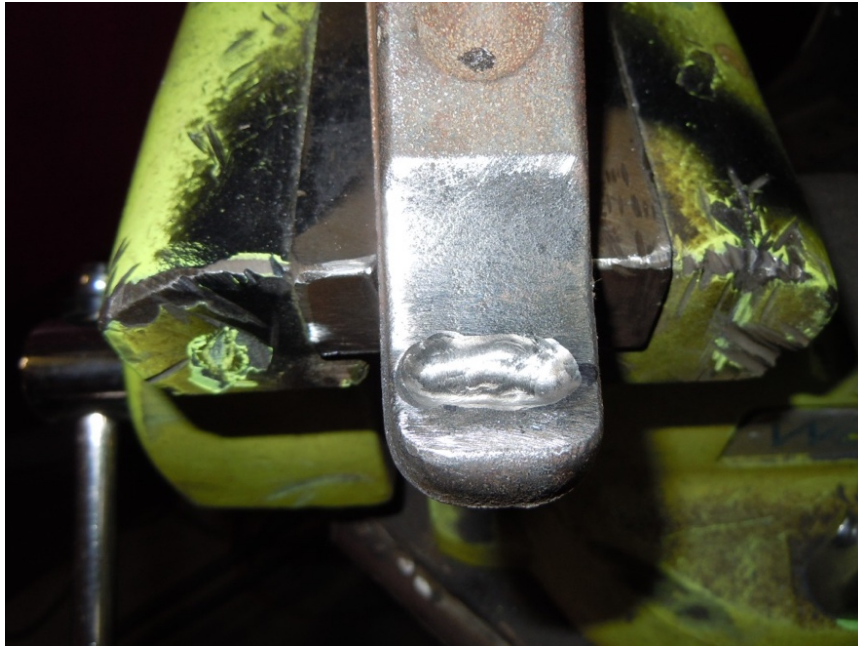
Figure 19: Use a carbide grinding bit to connect the 2 countersink spots in order to create an oval shaped pocket as shown. Now ready to install.
