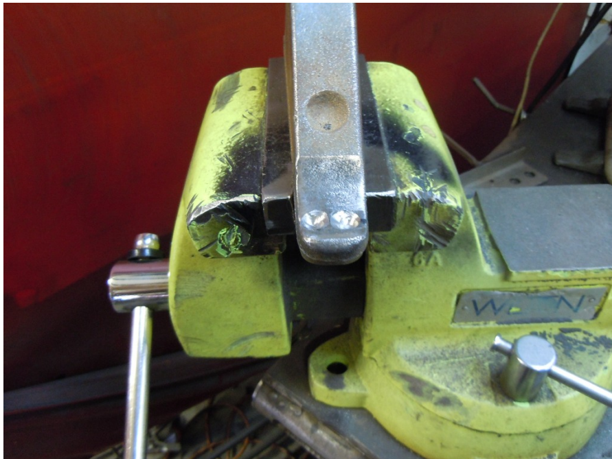
Figure 18: using a drill motor and 1/2" drill bit, drill only 1/8" deep from the tip so create 2 counter sink spots.
