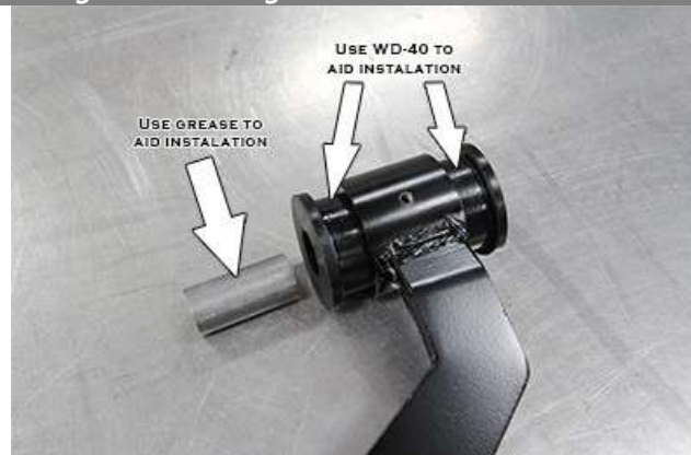
Figure 3: bushing and crush sleeve installation
