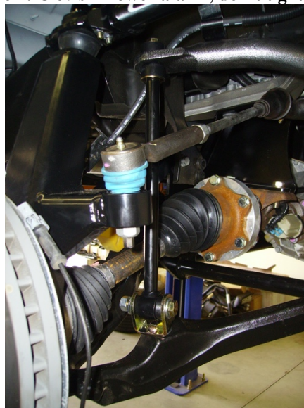
Figure 2: end link in place, clevis rotated so bushing relaxed, now tighten.
