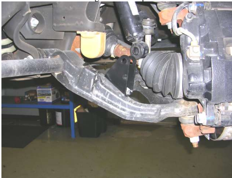
Figure 1: Cognito lower shock bracket installed.
