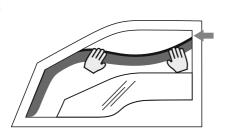
5. Bending the center part of the deflector outwards, insert the back part of the deflector into the channel, leaving a gap above it.
