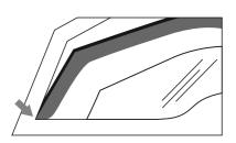
3. Place the front part of the deflector onto the lower frame of the window as shown in the picture.
