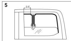
5. Bend the edge of the rubber seal from the front frame of the window by 2-3 inches. Place the fastening bracket in the channel and return the rubber seal to its original position.
