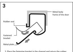
3. Place the fastening bracket in the channel and return the rubber seal to its original position.
