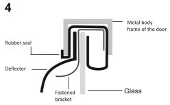
4. The picture demonstrates how to position the fastening bracket.
