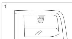
Make sure the car windows are clean and dry. Next, lower the side windows completely and clean the grease off the inner surface of the window channel with an alcohol wipe. 2
