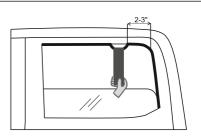
To position the fixture, bend the edge of the rubber seal from the back frame of the window by 2-3 inches by using a special metal plate as is shown in the picture.
