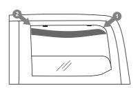
7. The deflector must be installed starting at the back. To do so, place the back part of the deflector frame into the channel and move the front part upwards. Position the entire deflector frame into the window channel, placing the frame between the fastening brackets and the rubber seal as is shown in the picture.
