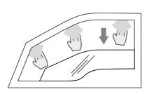
Make sure the car windows are clean and dry. Next, lower the side windows completely and clean the grease off the inner surface of the window channel with an alcohol wipe. 2
