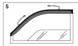
Totally remove the tape protective liner by pulling on free ends on the installed and aligned deflector(s) in sliding manner.
