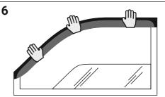
Tightly press the deflector to the installation point from one flange to another.
