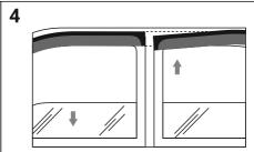
If you have 4 Piece Set, first attach FrontDriver Side Window Deflector and then the rear one. Align height of the rear deflector and front. Both parts should visually produce one straight line.
