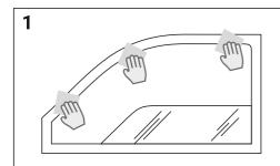
Wipe the installation point with the degrease prep-pad provided in the set (CAUTION! If you neglect this step deflectors won't be installed properly resulting in detaching from the vehicle door).
