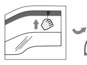
10. To ensure better installation of the deflector and better adhesion between the tape and the surface of the rubber seal, it is strongly recommended that you use the plastic blade, moving it slowly between the window's inner rubber seal and the deflector.
