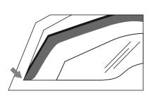
5. Lower the front part of the deflector onto the metal bracket as shown in the picture.
