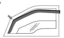
Shift the deflector forward, fitting the deflector frame into the channel completely. Make sure the deflector is placed above the lower window frame. 7
