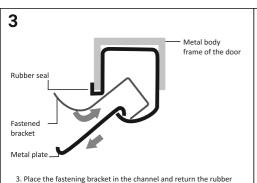
Place the fastening bracket in the channel and return the rubber seal to its original position.
