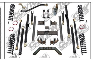
Note: Kits are the same except for the front center cross member. The 93-95 uses a round hole. The 96-98 uses a square hole with a ½ spacer plate. Note: Jeep Grand Cherokees with the full time 4 wheel drive transfer case may require custom modification of the cross member for proper driveshaft clearance. Most customers upgrade to a 231 or atlas transfer case which will solve this clearance issue.
