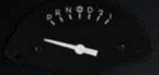
Optional Gear Indicator insert with or without overdrive (Without overdrive shown installed)
