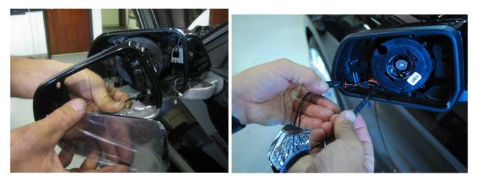
10. Connect heater wires to mirror. Route Signal wires as shown, below adjuster.
