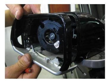
5. Remove the (3) T-15 Torx screws that secure the power adjuster to the mirror housing.
