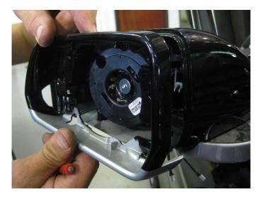
5. Remove the (3) T-15 Torx screws that secure the power adjuster to the mirror housing.
