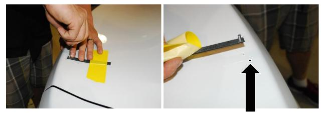
7. A.)Drill pilot holes with a 1/8" Drill. B.) Drill holes using 5/16" drill. NOTE: We strongly recommend using a Drill Stop to prevent any damage to the Taillights.
