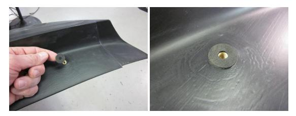
9. Apply 3M tape to the Spoiler as Shown in picture below. Clean the surface with the provided Alcohol Pack, and allow to dry completely. Apply the provided Adhesion Promoter, and allow to dry completely. Apply the provided 3M Acrylic Foam tape as shown in picture. HINT:
