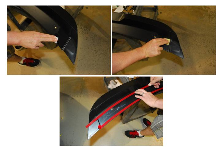
Temporarily place Outlaw Spoiler on Decklid and check alignment of holes. Open holes if necessary.
