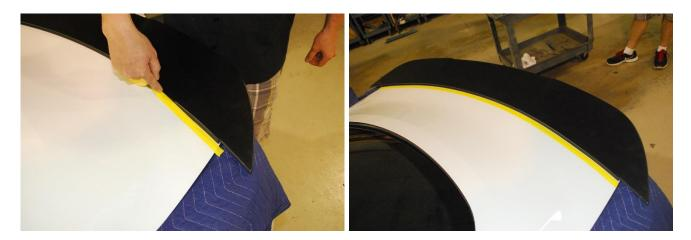
12. Clean Decklid with provided **Alcohol Pack**, and allow to dry completely. Apply the provided **Adhesion Promoter**, and allow to dry completely. Keep Adhesion Promoter about ¼" behind the masking tape. Remove Masking tape.
