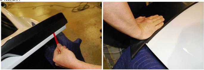
14. A.) Tighten the Spoiler Bolts. **Caution:** Do not over tighten. B.) Replace rubber grommets.
