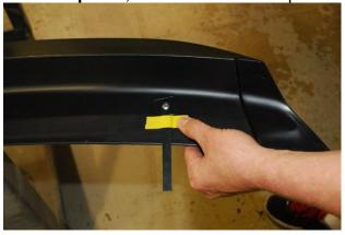
5. Place **Outlaw Spoiler** on Decklid. Make sure Spoiler is centered, and apply 2" Masking Tape to hold the Hole Locator Strips in place. Carefully remove Spoiler from Decklid, leaving the **Hole Locators** in place.
