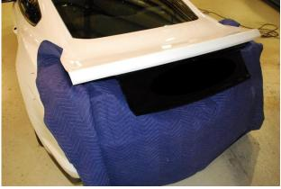
4. If car is equipped with Factory Spoiler, proceed to Step # 8. Insert the provided plastic **Hole Locator Strips** in the **Outlaw Spoiler**, secure with a small piece of Masking Tape.
