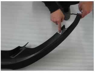
5. Apply the 1/4" **3M Acrylic Foam Tape** as shown, leaving "pull tabs" with the red backing.
