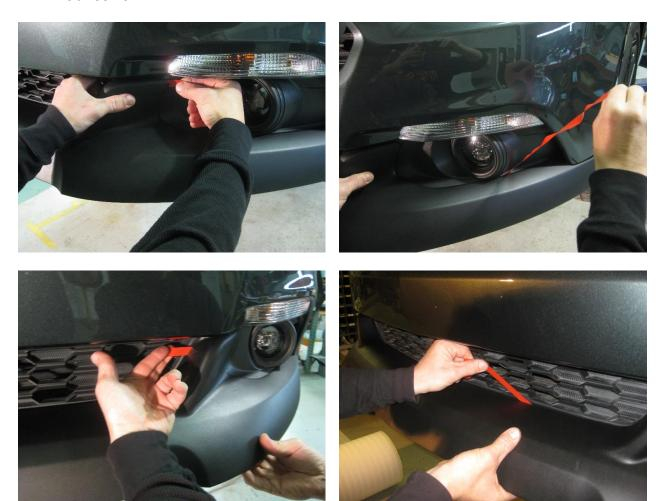
7. Reinstall the factory retainers removed in step #3, or use the provided Scrivets.
