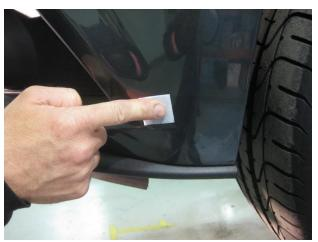
2. Install the provided **3M Acrylic Foam Tape** as shown in pictures below. *Note:* Apply tape about 1/8" away from fog light bezels and lower grille. Press tape firmly to activate the adhesive. *Important:* Create "pull tabs" with the red backing as shown.
