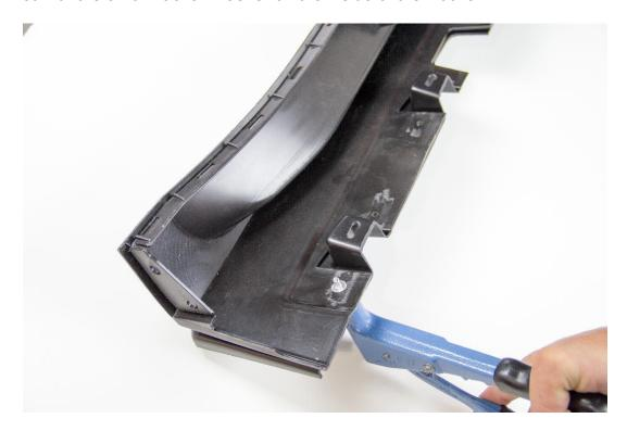
5. Align the last 3/16" Holes at the rear of the Rockers/Splitters. Install the Rivet with the 3/16" Backer Washer on the inside of the Rocker. **Note:** If holes don't line up perfectly, open with your drill. The heads of the rivets are oversized to accomadate.
