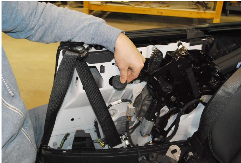
13. Remove 10mm window trim fastener.
