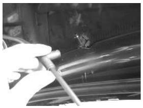
C) Remove fasteners that attach the hose to the hood with a fork tool. Cut the tape from the T shaped fastener with a razor blade and set aside for reuse.
