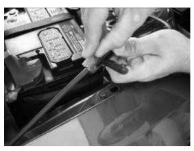
D) Separate the squirter hose at the tee fitting and set aside.
