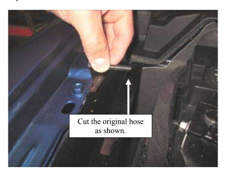
2) Route hose as shown under plastic cowl trim and behind the fender fastening point. Connect the factory hose to the new hose with the provided connector.
