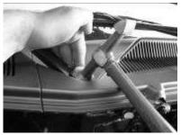
F) Remove Cowl Trim from vehicle. There are 4 plastic pieces to be removed, start with the small parts that are closest to the fenders. Use a short Phillips screwdriver to loosen the center of the fasteners and extract them with a fork tool. Once the 2 small parts are removed the large center parts can be removed, start with the passenger side.
