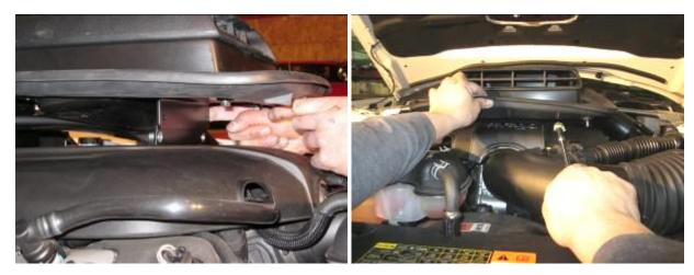
4. Attach the Air tube Adapter to the Upper Air tube. Do not tighten at this time.
