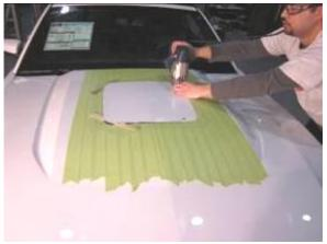
Hint: To help reduce excessive vibration, stop cutting at the half way point and place masking tape over the cut line to support the center piece of metal, or place paints sticks under the corners to prevent it from drooping into the engine bay.
