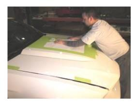
13. With a sharp razor blade or X-Acto Knife cut through template and tape, scoring the paint on the hood. Scoring the paint on the hood will help reduce the chance of paint flake during the cutting process.
