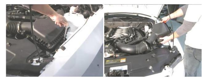
7. Close hood and mask off area where Shaker Opening will be cut out. Also add tape along the edge of the hood.
