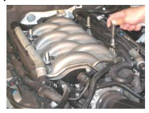
4. Reinstall the engine cover. The couplers are now visible through the drilled holes.
