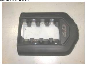
3. Install the 4 threaded couplers on the 4 fuel rail studs. Torque to 10.4 Nm or 7.8 lb-ft. Note: There are 2 different length couplers, 30mm and 33mm. The 30mm are to be used on the <u>forward</u> studs and the 33mm studs are to be used on the <u>rear</u> studs. Use a removable thread locker and torque to 10 Nm or 7.8 ft. lbs. DO NOT over tighten.
