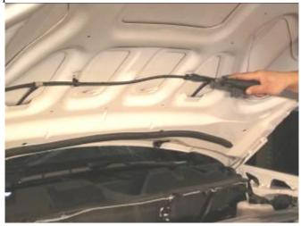
3. Disconnect them at the "T" (passenger side) and elbow (driver side). Hint: Twist the black plastic retainer counter clockwise to release.
