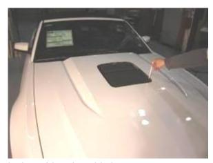
21. Cut opening in Hood Blanket with a sharp blade.
