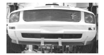
6. Using the Chin Spoiler fastener holes as a guide, drill the 10 fastener holes into the fascia.
