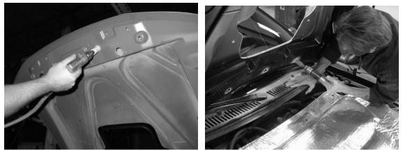
Note: DO NOT DRILL THROUGH THE HOOD OUTER WITH HOLE SAW!
