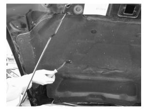
B) Close hood - Align template with hood feature lines as noted on template. Tape template securely to outside hood surface.
