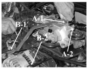
B) Repeat step A with bolts A-2 and B-2. Install Ball Studs onto center hole of brackets.
