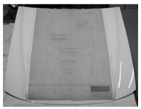
Note: During the drilling and cutting process, elevate hood far enough to ensure no damage will occur to engine components.
