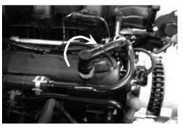
31. Bend tabs for the engine ground and wiring harness on the firewall down.
