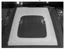
10. Drill a starter hole for Shaker opening with a 1" Holesaw. Cut Shaker opening following the tape outline.
