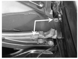
B) Route the new Hose down the bottom side of the wiper arms securing the Hoses in the Clips as you go.
