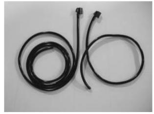
D) Clip the Squirter Nozzle with **63" Hose** onto the Driver Side wiper arm and the Squirter Nozzle with **26" Hose** onto the Passenger Side wiper arm, as shown below.
