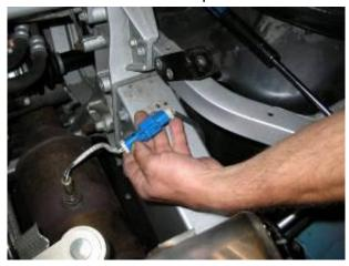
**9. Remove Ground Wires from Horns**. Remove the 10 mm bolts that secure the ground wires on both Frame Horns.
