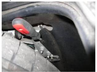
**11.Remove License Plate to gain access to the Upper Mesh Panel fasteners**. Remove the (4) T-27 Fasteners and remove license plate.
