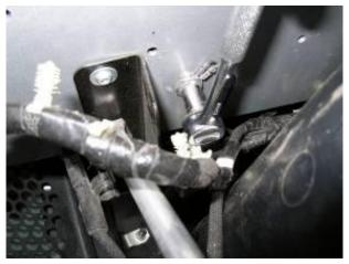
**10.Remove push pin fastener from wheel well liner on driver and passenger side.**There is 1 push pin fastener on both driver and passenger sides that secures the wheel liner to the Frame Horn. Remove from both sides. 2 new push pins are included for reinstalling.
