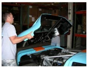
**3.** Remove Air Box to gain access to exhaust tip clamps. Loosen the 8mm hose clamp. Unplug Mass Air Sensor. Remove the (2) 10mm mounting blots. Remove Air Box from vehicle.
