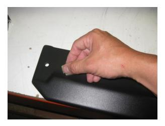
5. Locate 1 of the 2 larger diameter push pins (CDC# 116020) from the hardware package and insert though larger hole in rear of Splitter. Peel about 3" of the red backing and temporarily tape with masking tape as shown, at front and rear of Rocker.
