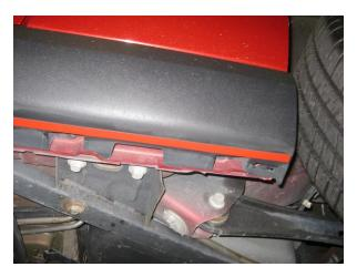
4. Apply Adhesion Promoter to Splitter as shown in pic. **NOTE:** Apply Promoter where tape will contact the Splitter.
