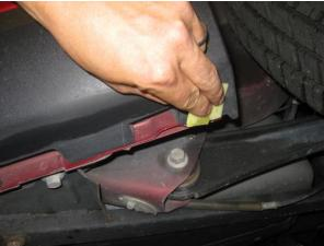
3. Apply 3M tape to bottom side of Rocker. **NOTE:** Use the rectangle cutouts in the bottom of the Rocker as a guide to place the 3M tape.
