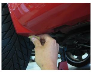
4. Apply the 3M tape as shown below. **NOTE:** Apply the tape approximately 1/16" inboard of the corner of the Rocker Panel.
