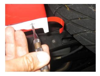
8. Align template as shown at front of Rocker. Mark the Rocker with a center punch.
