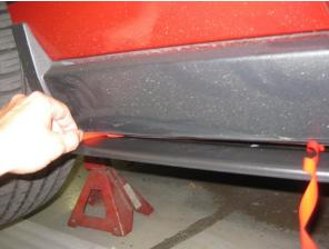
8. Using the Splitter as a drill guide, drill the remaining ¼" holes and install push pins. Repeat the process on the opposite side of the car.
