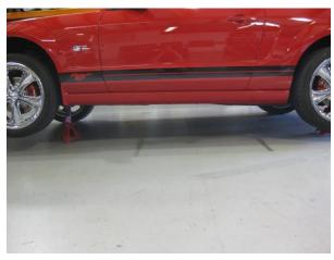
2. Clean the bottom side of the Rocker Panel with the supplied Isopropyl Alcohol Pad. **NOTE:** You may need to first use a damp cloth to clean the Rocker Panel if it is excessively dirty. Make sure it's dry before using the Alcohol Pad.
