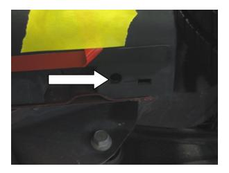
7. This step is easier with the help of a friend. Hold up the front of the Splitter so that the inside radius fits the Rocker well, and looks parallel to the Rocker. Peel the red backing and press the Splitter firmly into position against the bottom of the Rocker. **Caution:** If your car is on jack stands, use extreme caution.
