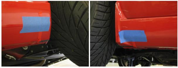
11. Insert 1 of the included push pin fasteners (CDC# 65003) through the most rearward hole in the Splitter and into the hole previously drilled in the Rocker. Do the same at the front of the Rocker.
