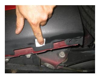
2. Apply Adhesion Promoter to the bottom side of the Rocker as shown. Allow sufficient time to dry.
