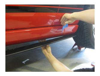
12. Peel the remaining red backing while firmly pressing the Splitter up to the bottom of the Rocker.
