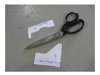
7. Align template as shown at rear of Rocker. Mark the Rocker with a center punch.
