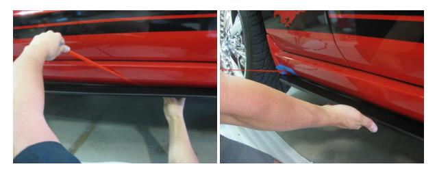
13. Using the Splitter as a drill guide, drill the remaining ½" holes and install push pins. **NOTE:** There are 2 large diameter push pins that are not used for 2005-2009 installation. Repeat the process on the opposite side of the car.
