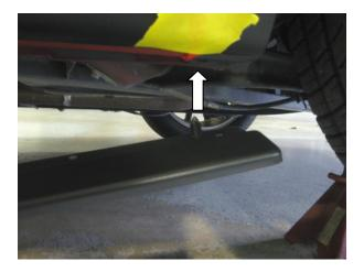
6. Use the hole in the pic to help locate the Splitter in the correct location.
