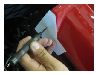
9. Drill both front and rear locations with ¼" drill. **NOTE:** If you did not jack the car up, you will need a right angle, or 90 degree drill. It's ok if you drill through the 3M tape.
