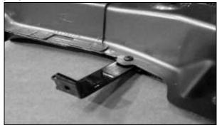
16. Install one *U-Nut/Clip* onto both *Short L Brackets*, on the side of the L Bracket that has the slotted hole. Face the threaded side of the clip towards the inside of the "L".
