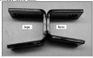
9. Install the four *U-Bracket & Clip Assemblies* to fascia through the existing four slots that secure the lower edge of the factory grille. From the backside of the slots, feed *U-Bracket Assembly* (starting with leg that does not have the *U-Nut*) through each slot as shown below.
