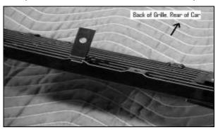
18. Place Billet Grille onto fascia and start all six mounting screws through Grille Mount Tabs into brackets, use thread locker on all screws. Just snug screws at this time.
