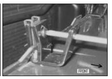
10. Install a *Clamp Bracket* onto each of the *U-Brackets* and Secure with a Phillips Head screw (supplied) as shown above, use thread locker on screws.
