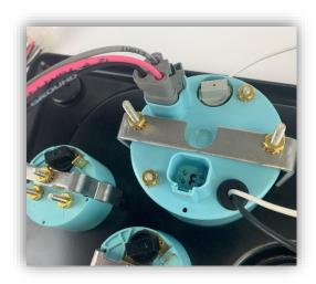
The GPS Plug-and-Play Antenna (included) plugs directly into the back of the speedometer. The black and white wires shown on the back of the speedometer are for TRIP / RESET. Install push button switch (included) between these two wires.
