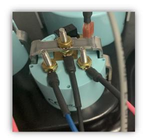
The oil pressure gauge will have 4 wires connecting to it:
