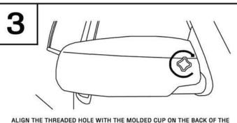
ALIGN THE THREADED HOLE WITH THE MOLDED CUP ON THE BACK OF THE WEDGE. SCREW KNOB THROUGH RAISED HOLE ON BACK OF TOWING MIRROR. TIGHTEN SECURELY.
