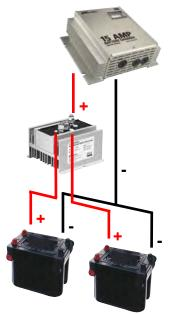
12V DC Charging System including (from top to bottom): battery charger, battery isolator and battery bank.
