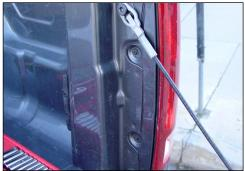
Remove the two torque screws that hold the taillights assembly to the truck.
