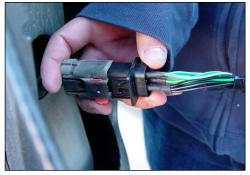
Plug in the new L.E.D taillights assembly to the stock wire harness.
