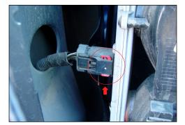
Pull the red clip down to remove the plug from stock taillights assembly.
