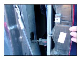
Pull the taillights assembly straight out to remove.
