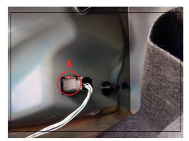
Pull the red clip out and disconnect the plug from the housing. Pull the taillight straight out.
