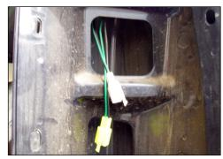
Install the resistor boxes in a location out of the way of the taillight housing.
