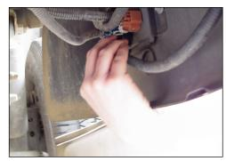
Connect the new wire harness to the circuit board underneath the vehicle. Make sure all functions are working properly before driving.
