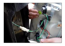
Connect the resistors to the wire harness. Make sure they are plugged in securely.
