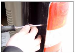
Remove the two phillip head screws that hold the taillight in place. Pull the taillights straight out.
