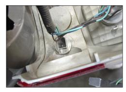
Reinstall the side marker light into the new housing. Connect the resistor box to the wire harness.
