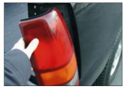
Once the screws are removed, you will be able to pull tail lens straight out.
