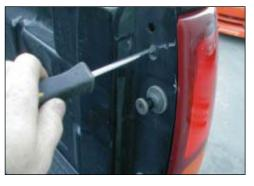
Open tailgate and remove the phillips head screws located inside the tail gate area.
