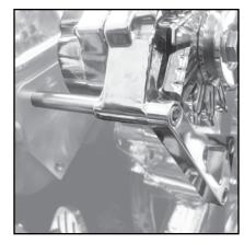
4. Mount the 1 5/8" adjustment rod to the front top left side of the water pump using one 3/8" x 1" SHCS bolt. On the other end of the 1 5/8" rod mount it on the backside of the alternator with a 3/8" mounting. For the best results, when finished adjust the rod and make sure all bolts are securely tightened.
