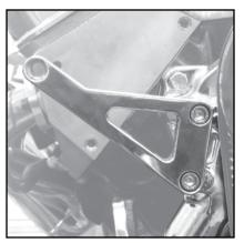
3. Using one 3/8"-16 x 6" SHCS bolt, insert into the alternator with a 2 3/4" diameter mounting using 3.250" spacer between the alternator and the hole on the upper left passenger side head. KEEP THE BOLT LOOSE FOR ADJUSTMENT FROM THE ROD.
