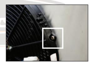
Attach fan shroud, with fan attached, to radiator by mounting to the holes that were drilled into the metal lips in Step 2. Use preferred mounting method (rivets pictured).
