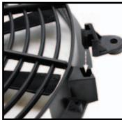
Slide nylon tie through fan mounting hole and into radiator fin hole with foam mounting pad placed inbetween. Insert tie through lock tab clip on other side until it is snug against radiator. Cut excess nylon tie as necessary.
