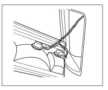
**1.** Remove both tail light assemblies and locate the vehicle's wiring harness. There will be connection points on each side of the vehicle matching the ends of the T-connector adapter.
