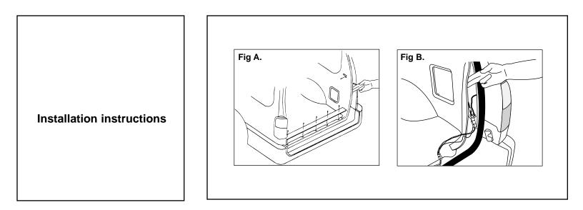
**1.** Open the rear door of the vehicle and remove the five screws attaching the threshold panel.
