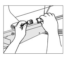
**1.** Locate the vehicle's taillight wiring harness along the inside of the left rear frame rail. This harness will have a connection point with connectors matching the ends of the T-connector adapter.
