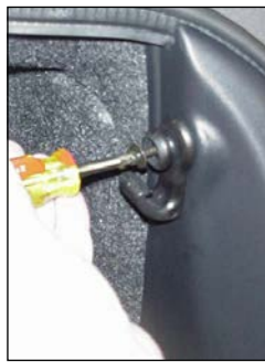
REMOVE CARGO NET LATCH FOR REMOVAL OF TRIM PANELS.
