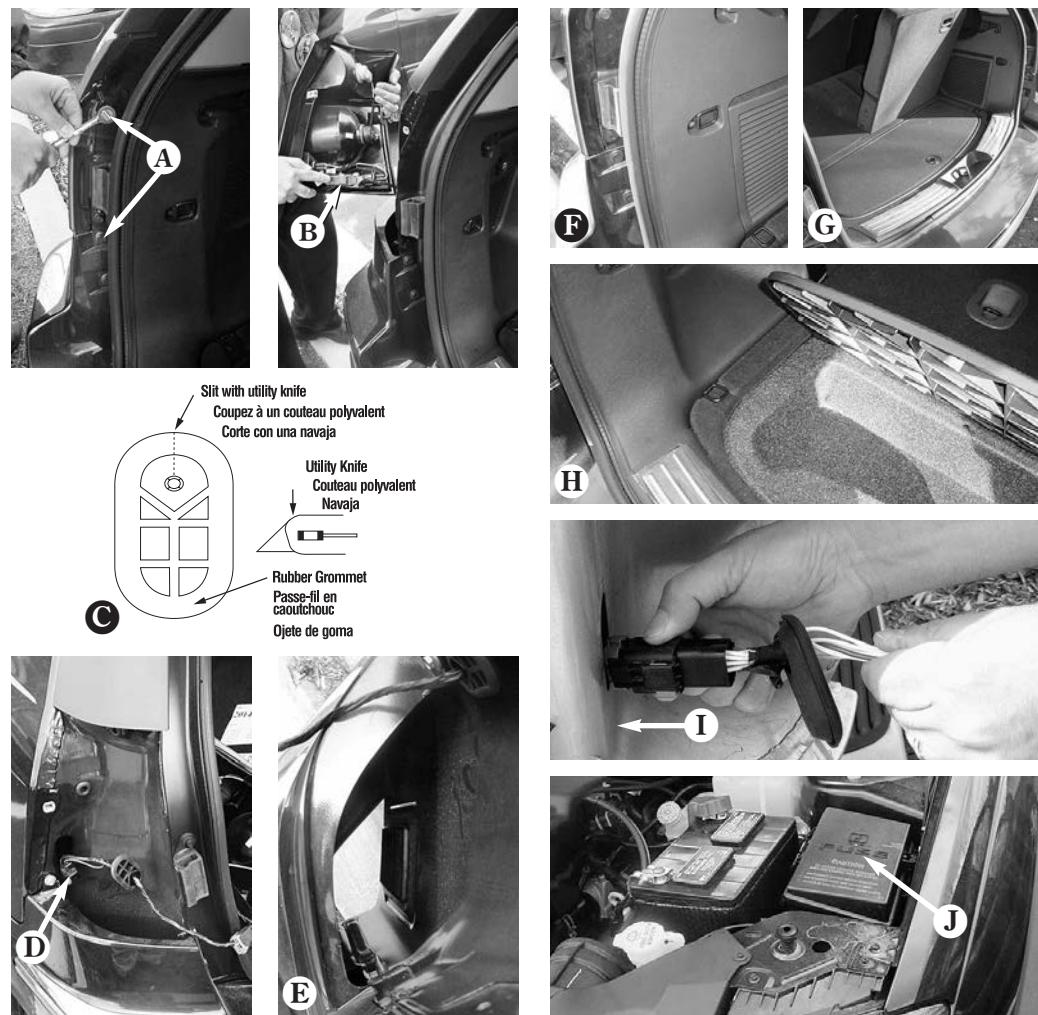
1. Open the tailgate and remove the vehicle's taillight assemblies by removing the two 10mm hex head bolts on each side. Carefully pry the housings away from the vehicle, being careful not to break the alignment tabs **A** & **B**.
