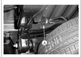
Locate the vehicle's tail light wiring harness underneath the truck bed near the driver's side frame rail (). This harness will have a connection point with connectors matching the ends of the T-connector harness.
