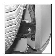
**1.** Locate tow vehicle's trailer harness connector. This harness is located under the vehicle, behind the rear bumper, on the passenger's side of the vehicle.
