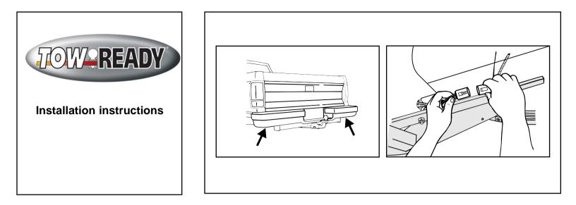
**1.** Locate the vehicle's factory tow harness connector behind the bumper. (Ranger left side), (Explorer right side) This harness will have a connector that will mate to the end of the tow plug.
