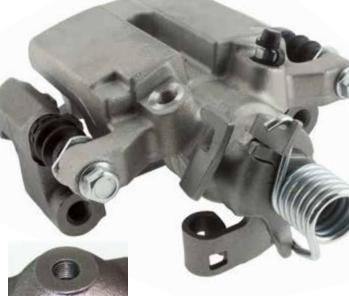
Where necessary Centric Parts remanufactured caliper hydraulic connections are knurled to ensure proper sealing of the brake line to the caliper body, eliminating leaks. Centric uses caliper-specific fixtures during the knurling process mating surface.
