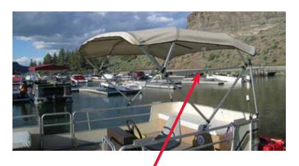
Free Standing Pontoon Top has a center cross strut for stability rather than front hold-down straps.
