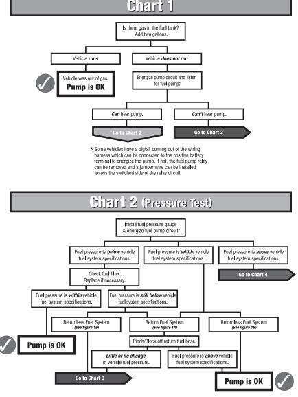
\* Make sure the pressure gauge you use is rated for the specified fuel system pressure of the vehicle. Most vehicles will have a Schrader valve on the fuel rail to hook a pressure gauge to. If it does not, refer to Figures 1A & 1B for correct gauge location or refer to the OE service manual for correct gauge connection.
