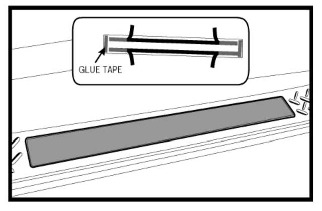
4. Remove the release paper of the double-sided tape by pulling it, and securely install the Front Plate and the Rear Plate. Press the sill plate firmly to tighten the application.
