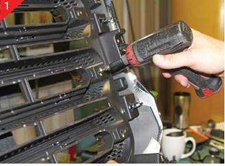
Remove stock shell and place on protective work surface. Next remove (6) screws from the backside holding chrome accents in place to the face of the stock grille shell.
