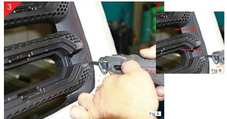
Next you will be cutting the center portion of the stock grille shell. Starting in the lower right hand corner follow around as shown above using an air saw or cut-off wheel. There is a molded line in the grille shell to follow shown above in RED. (Fig B shows acutal line). You will cut both the driver and passernger side of the grille shell then move on to the top and bottom portion.
