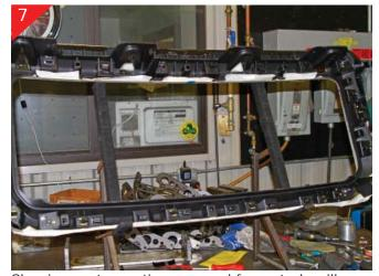
Showing center portion removed from stock grille shell.
