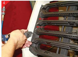
Continued cutting of the passenger side of the grille shell again following the line in the grille shell.
