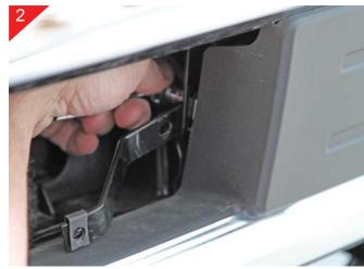
Next locate and remove the stock 10mm bolts located on each side of the bumper opening. Next attach brackets using the just removed 10mm bolts as shown above.
