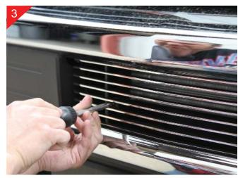
Next place billet grille into bumper opening and center. Attach billet grille to the already placed brackets using the supplied 10-24 x 1" bolts.
