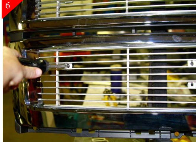
Turn grill shell face up. Place Billet grilles into opening and center. Secure in place using the supplied 10-24 x 1" Phillips head bolts.
