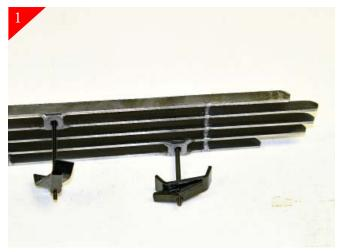
Start by Attaching brackets loosely to billet grille in order for you to rotate the brackets around so they fit through the opening in the bumper. Place bolt through the mounting tabs followed by "C" bracket and toggle wing as shown above.
